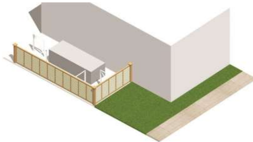
Figure 10-19 Ground/Wall-Mounted Mechanical Unit Screening
