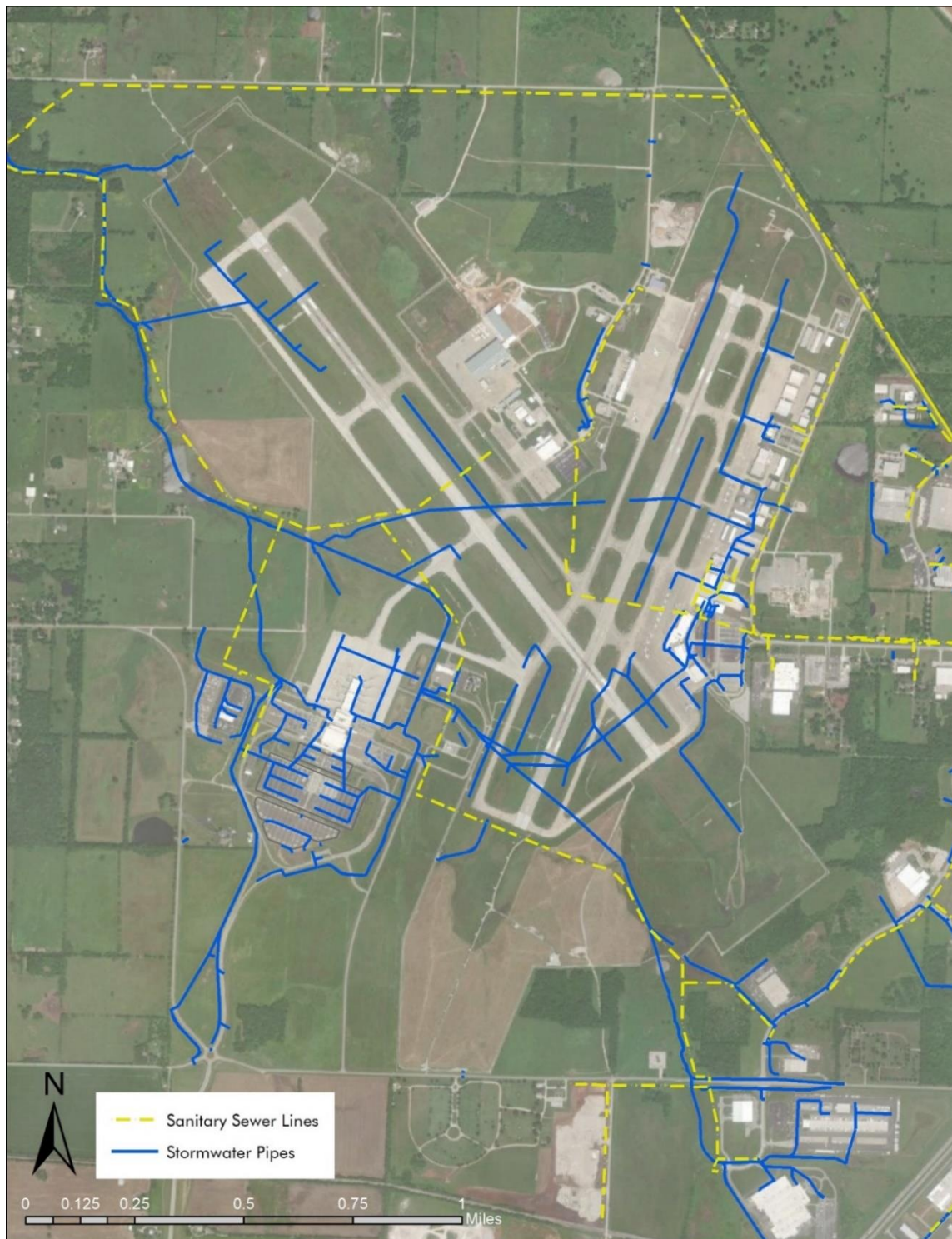
Exhibit 1.4-10: Sanitary Sewer and Storm Water Infrastructure near SGF
