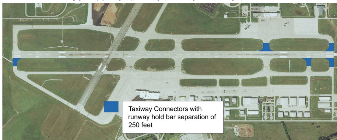
FIGURE 4-5 - RUNWAY HOLD BAR SEPARATION
