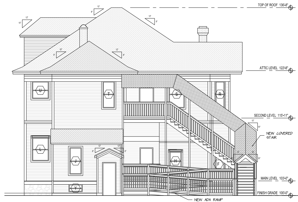
1 SOUTH ELEVATION @ REAR ENTRY/EXIT 1/4" = 1'-0"
