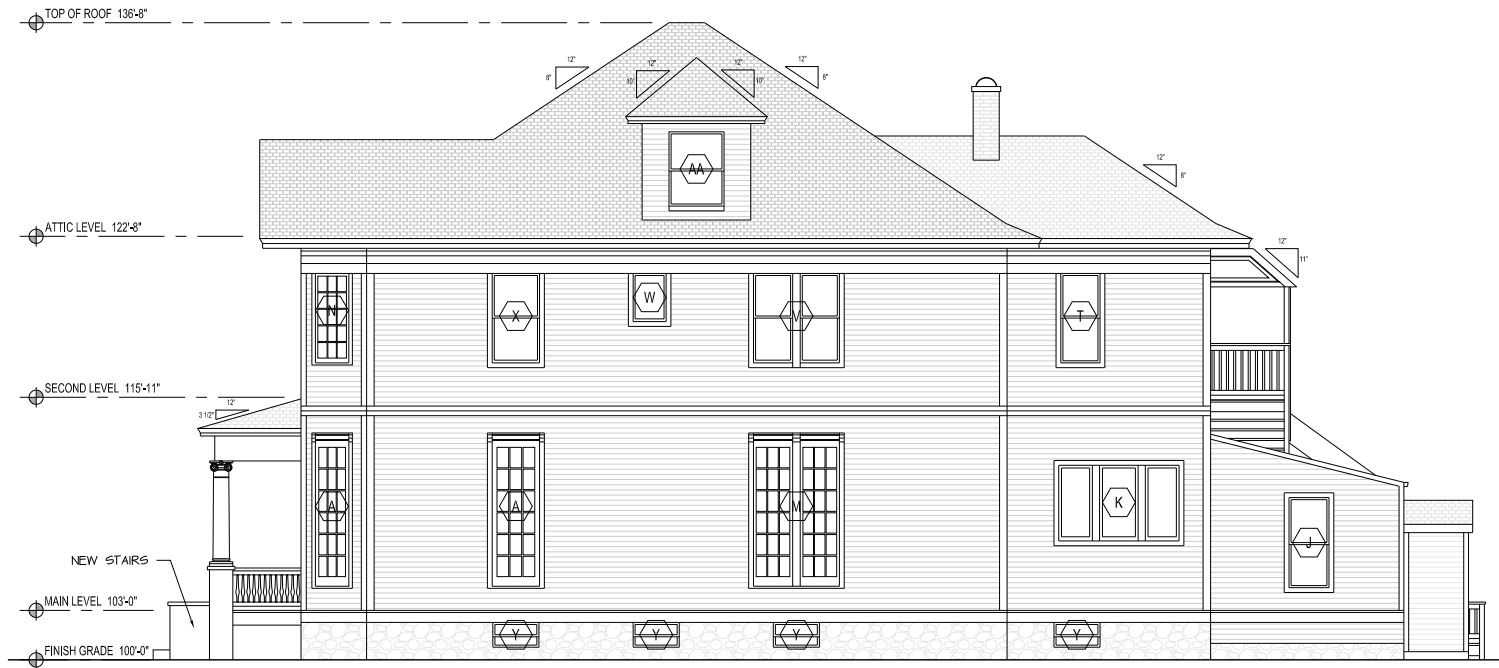
3 WEST ELEVATION @ REAR PORCH 1/4" = 1'-0"
