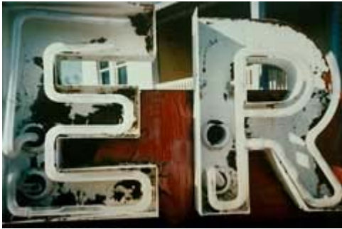
These tubes in this amusement park's sign were broken and the surrounding "metal cans" needed work also. See below. Photo: Stan Fowler.
