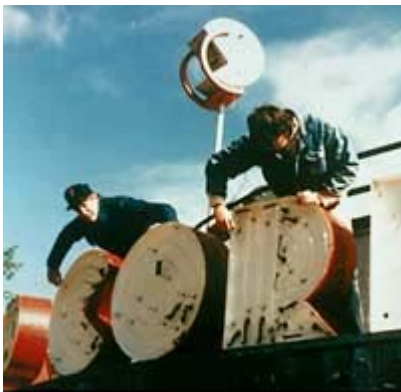
Neon fabricators are installing the new tubing in the repaired and remounted cans. Photo: Larry Kanter.
