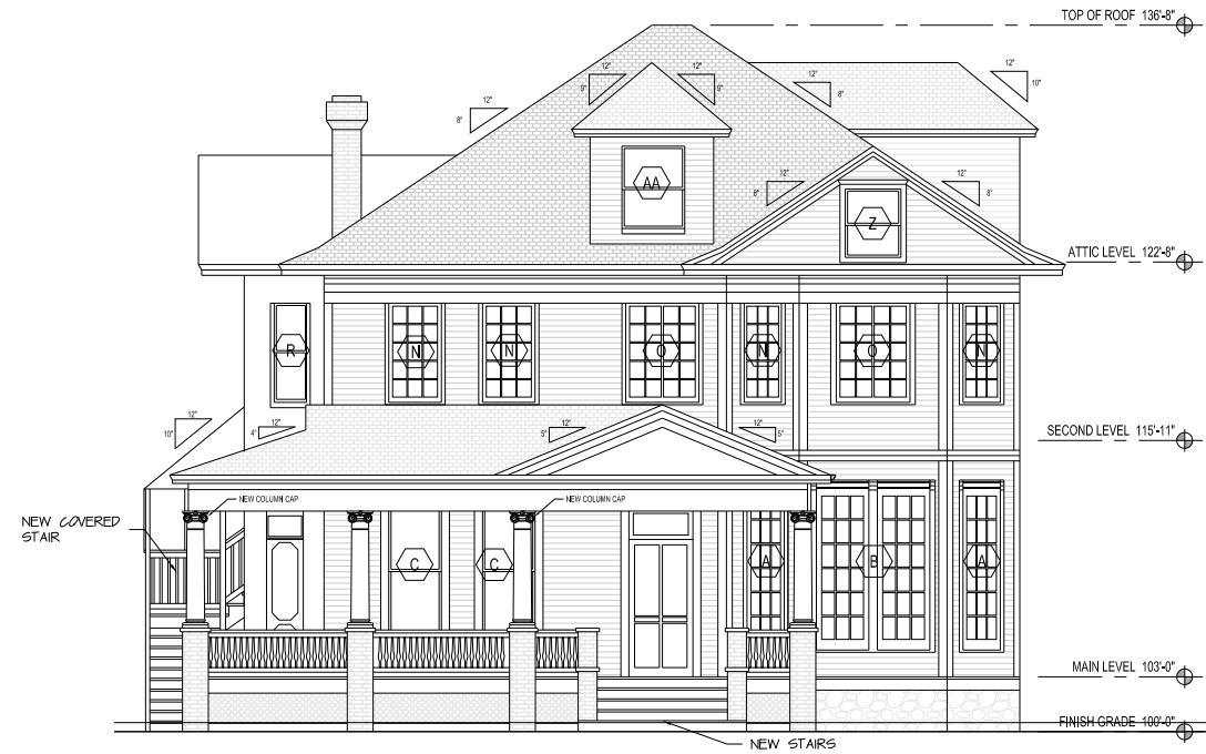
4 NORTH ELEVATION @ FRONT PORCH 1/4" = 1'-0"
