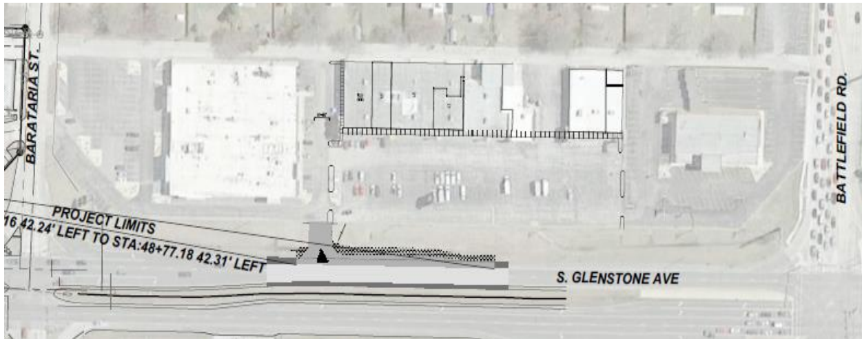
Figure 6: Depiction of proposed right in/right out turn lane access improvements to the Study Area south of Barataria Street.
