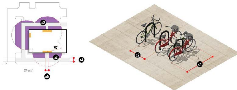
Figure 10-40 Off-street Bicycle Parking
