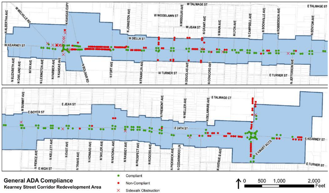
Figure 10 – General ADA Compliance
